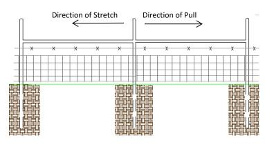
Single H brace end panel assemblies are required where fences end and on both sides of gate opening where the pull is only one direction.
