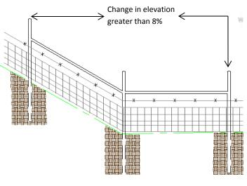
Double H brace corner assemblies are required at all points where the fence alignment has a change of 20 degrees or more and the pull is from two directions.
